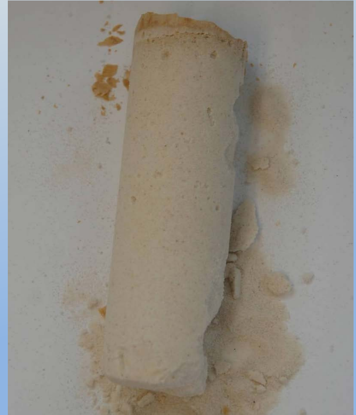
Fully-Cemented Specimen (Qabany et al. 2012)
