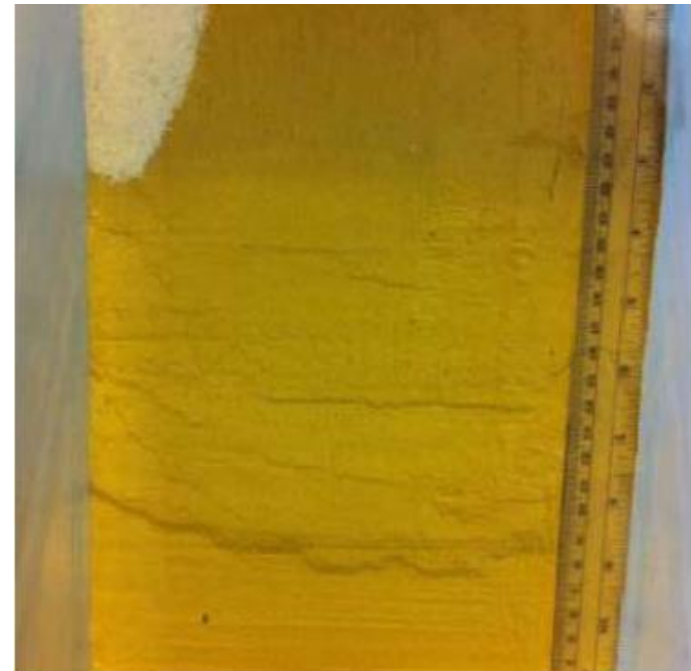
Observed rupture on surface of embankment in Test 10
