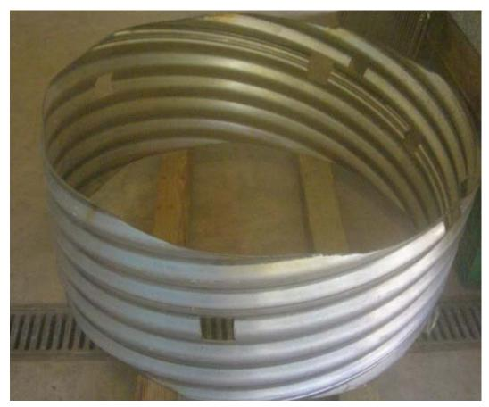
Figure 14. Pipe #2014-08-037 – 36" section of pipe. Five areas had visible damage, and samples were removed for metallographic analysis.
