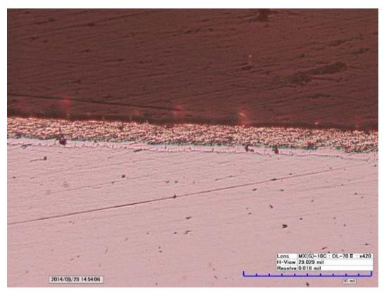
Figure 26. Pipe #2014-09-008 – Cross section of the control sample showing no visible damage to the aluminum layer; 420x
