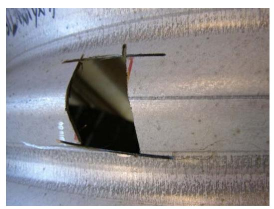
Figure 74. #2014-09-018 – Close up of rolling marks on top of the corrugation showing visible markings on the pipe.
