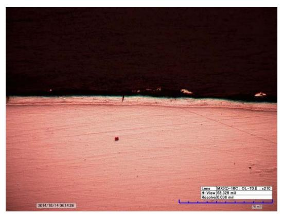
Figure 75. #2014-09-018 – Cross section of the rolling mark area shows no damage to the aluminized layer. 210x
