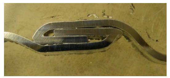
Figure 79. #2014-09-018 – Low magnification of the Lock Joint.
