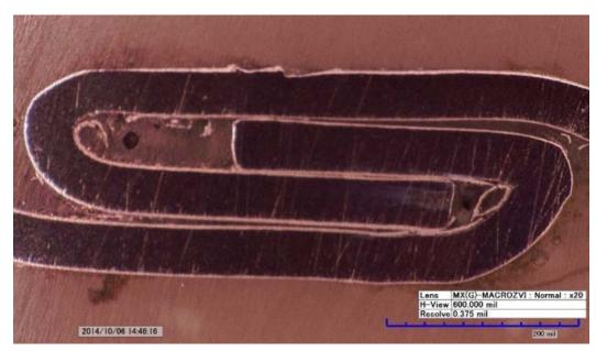
Figure 68. #2014-09-017 – Low magnification of the lock joint. There is apparent damage to the aluminum layer on the exterior, as well as the common damage in the folds to the aluminum layer. 20x
