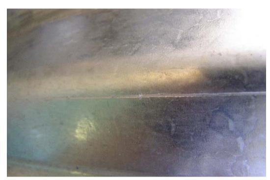
Figure 4. Pipe #2014-08-036 – Close up of a deep scratch on the corrugation. Visible damage to the aluminum coating is seen.
