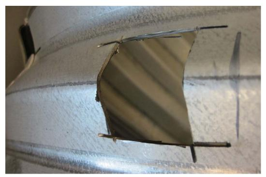
Figure 87. #2014-09-046 – Close up of rolling marks on top of the corrugation showing visible markings on the pipe.
