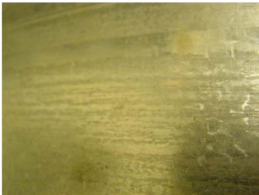
Figure 36. Pipe #2014-09-009 – Close up of the control sample showing no visible damage to the aluminum layer.
