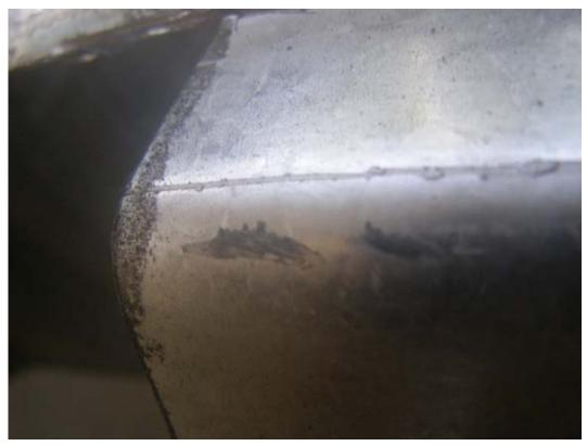
Figure 7. Pipe #2014-08-036 – Close up of gouges in the pipe. This shows visible damage.
