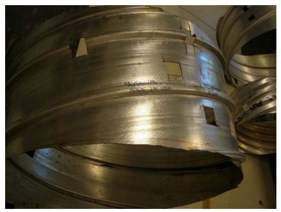
Figure 35. Pipe #2014-09-009 – 36" section of pipe. No visible damage to the aluminum coating. Multiple rolling marks on the corrugations.
