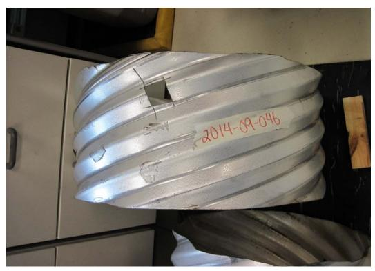
Figure 84. #2014-09-046 – 24" section of pipe. Two areas had visible damage, and samples were removed for metallographic analysis.
