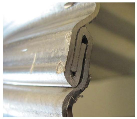
Figure 92. #2014-09-046 - Close up of the lock seam.
