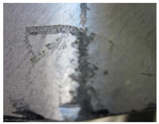
Figure 89. #2014-09-046 – Close up of scrape marks on the corrugation.
