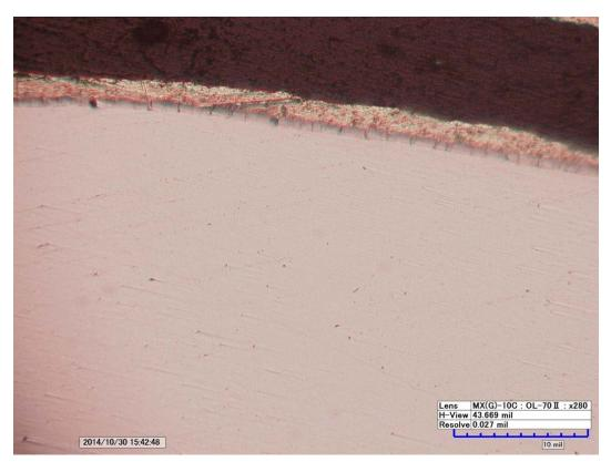
Figure 95. #2014-09-046 - Cross section of the lock joint showing no visible damage to the aluminum or inner metallic layer. 280x
