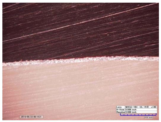
Figure 28. Pipe #2014-09-008 – Cross section of rolling mark area showing no visible damage to the aluminum layer. 140x
