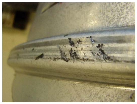
Figure 103. #2014-10-02 – Close up of scuff or scrape marks on the corrugation.
