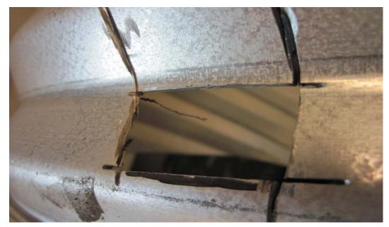
Figure 85. #2014-09-046 – Close up of a control sample. This shows no visible damage.
