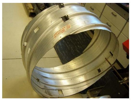
Figure 24. Pipe #2014-09-008 – 36" section of pipe. No visible damage to the aluminum coating. Multiple rolling marks on the corrugations.
