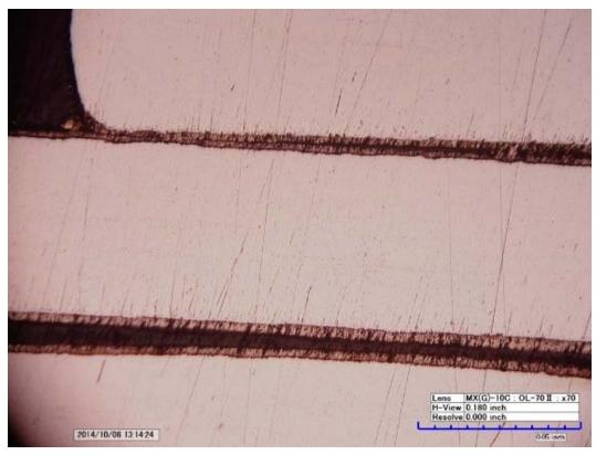
Figure 69. #2014-09-017 – The center of the lock joint shows no visible damage to the aluminum layer. 70x
