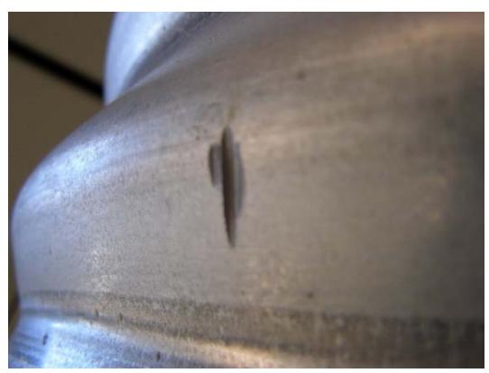
Figure 76. #2014-09-018 – Close up of a gouge or cut in the pipe.
