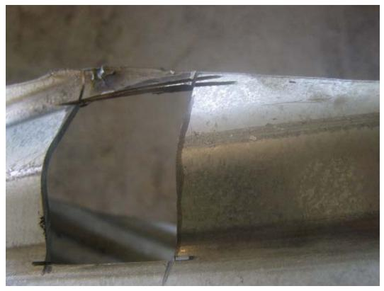
Figure 17. Pipe #2014-08-037 – Close up of a rolling mark showing visible markings on the exterior.
