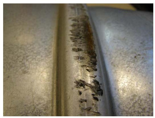
Figure 106. #2014-10-02 – Close up of scuff or scrape marks on the corrugation.
