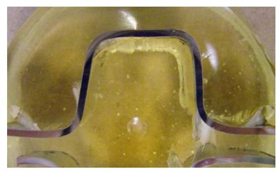
Figure 30. Pipe #2014-09-008 – Low magnification cross section of the rolling marks.
