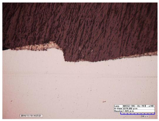
Figure 70. #2014-09-017 – Cross section of the lock joint showing damage on the top surface to the aluminum layer, inner metallic layer and the steel substrate. 140x
