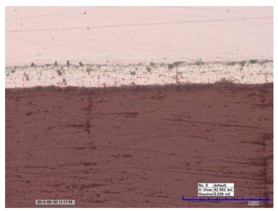
Figure 43. Pipe #2014-09-009 – Cross section of rolling mark area under further magnification showing no visible damage to the aluminum layer; 420x
