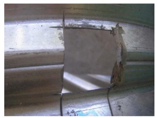
Figure 10. Pipe #2014-08-036 – Close up of the lock seam. There was no visible damage.
