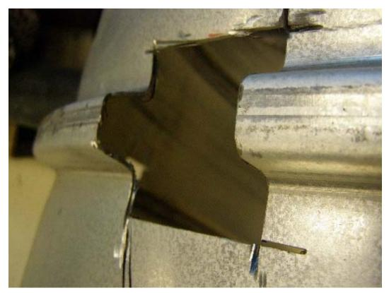
Figure 101. #2014-10-02 – Close up of rolling marks on top of the corrugation showing visible markings on the pipe.
