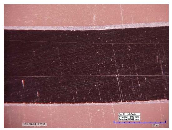
Figure 42. Pipe #2014-09-009 – Cross section of rolling mark area showing no visible damage to the aluminum layer. 70x
