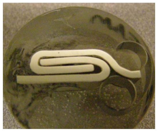
Figure 112. #2014-10-02 – Low magnification cross section of the lock joint showing no visible damage to the aluminum layer.
