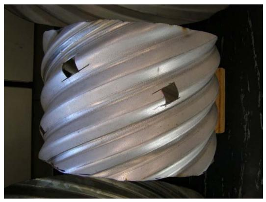
Figure 71. #2014-09-018 – 36" section of pipe. One area had visible damage, and samples were removed for metallographic analysis
