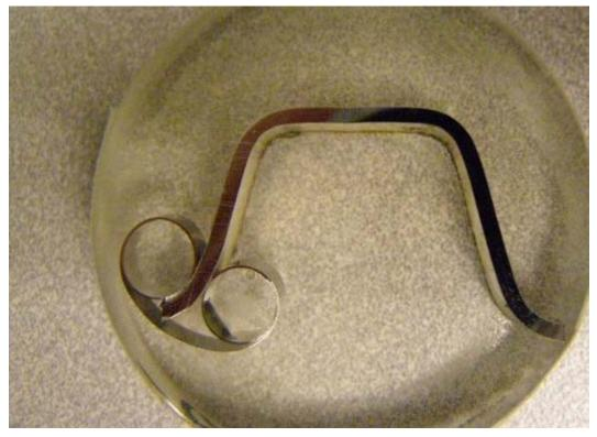
Figure 104. #2014-10-02 – Low magnification cross section of the corrugation at locations of scrapes.
