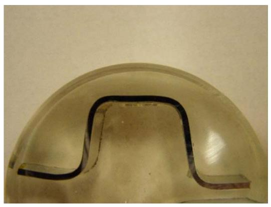
Figure 45. Pipe #2014-09-009 – Low magnification cross section of the corrugation at locations of scrapes.
