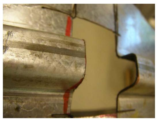
Figure 38. Pipe #2014-09-009 – Close up of rolling marks on top of the corrugation showing visible markings on the pipe.
