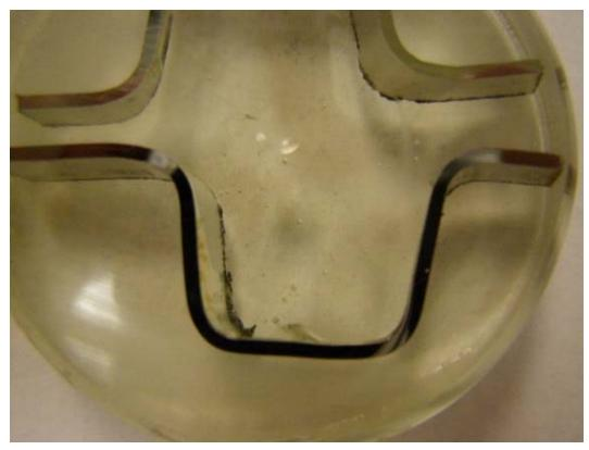
Figure 39. Pipe #2014-09-009 – Low magnification cross section of the rolling marks.
