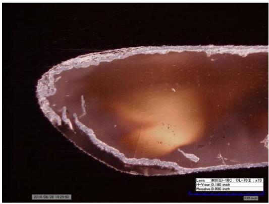
Figure 12. Pipe #2014-08-036 – The lock joint was examined under further magnification after additional polishing was performed. A clear separation of the aluminum layer is seen. 70x
