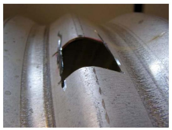
Figure 63. #2014-09-017 – Close up of rolling marks on top of the corrugation showing visible markings on the pipe.
