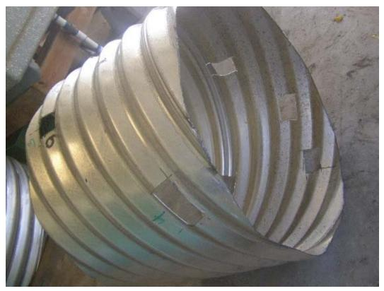
Figure 1. Pipe #2014-08-036 – 24" section of pipe. Eleven areas had visible damage, samples were removed for metallographic analysis
