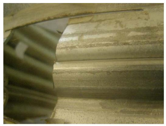
Figure 21. Pipe #2014-08-037 – Close up of the lock seam. There was no visible damage.
