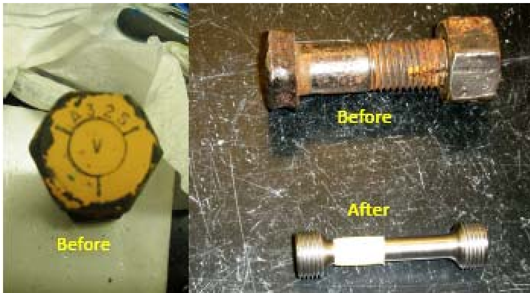
Figure 1 Photo of typical bolt prior to and subsequent to coupon fabrication
