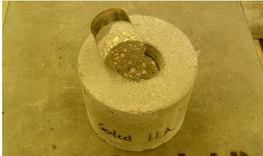
Figure 17: Direct tensile specimen
