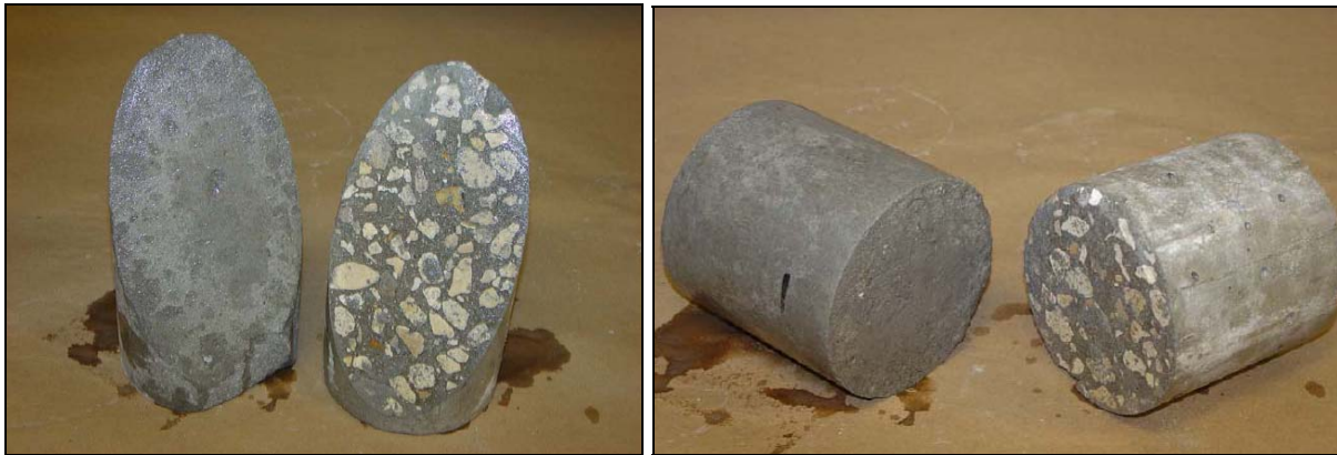
Figure 16: Slant shear testing (left) and Iowa shear testing (right)
