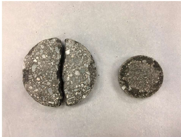
Figure 4. Comparison of 6-inch vs. 4-inch Diameter Specimens after Cantabro Loss Testing
