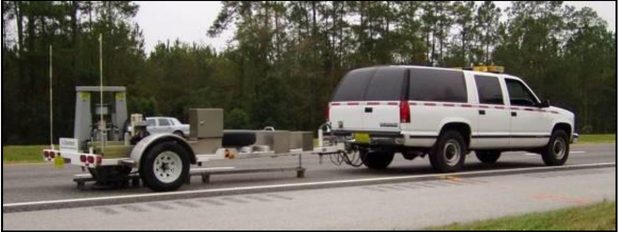
FIGURE 3. Falling Weight Deflectometer
