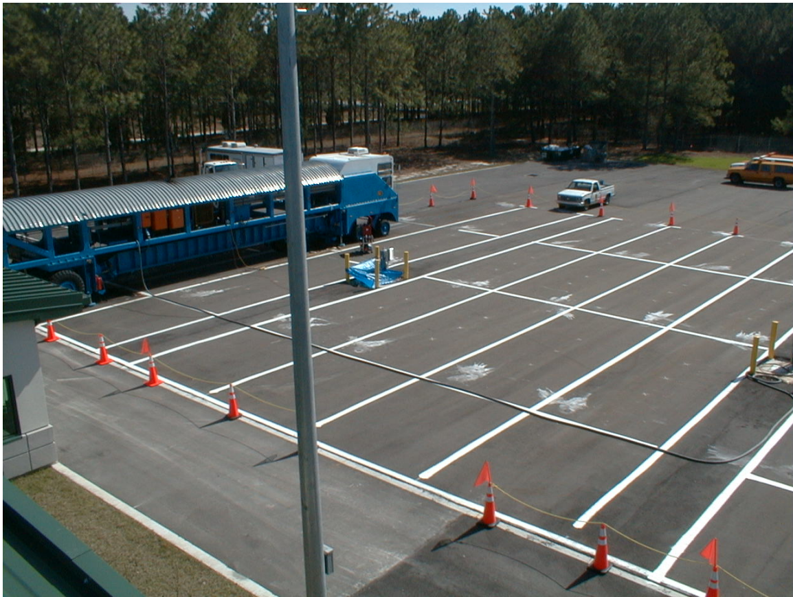
FIGURE 1. HVS and test tracks.
