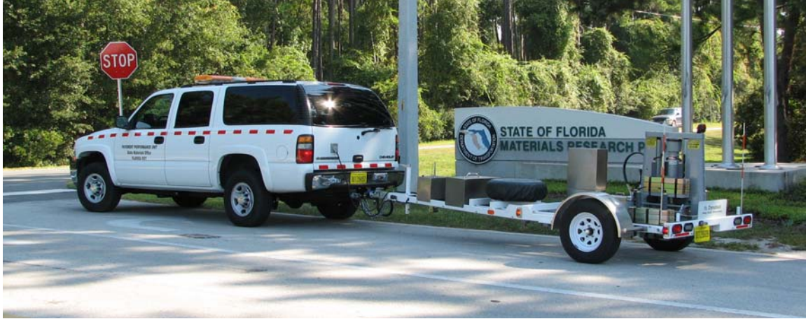
Figure 4. Falling Weight Deflectometer
