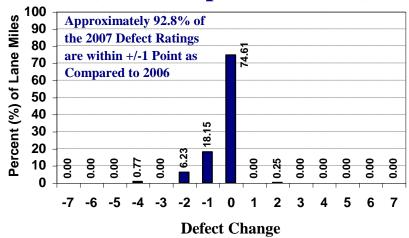
NEGATIVE VALUES ARE INDICATIVE OF THE DETERIORATION IN THE PAVEMENT AND/OR THE VARIABILITY IN THE DATA COLLECTION PROCESS
