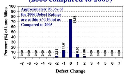
NEGATIVE VALUES ARE INDICATIVE OF THE DETERIORATION IN THE PAVEMENT AND/OR THE VARIABILITY IN THE DATA COLLECTION PROCESS
