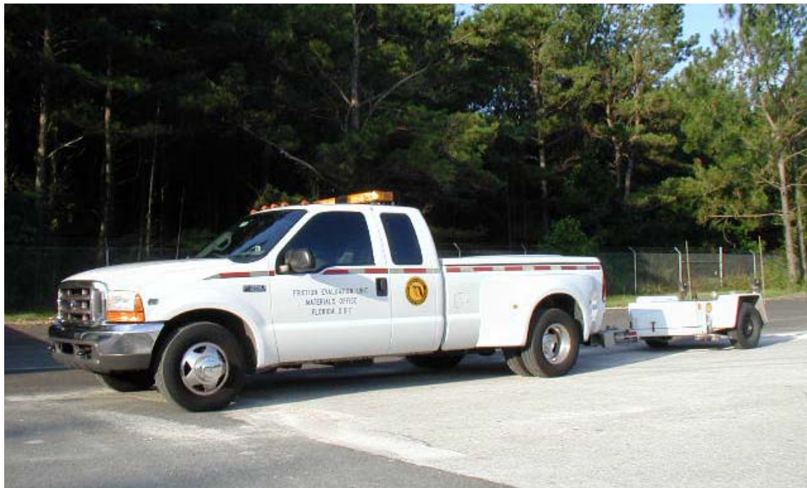
Figure 2 Photographic illustration of a FDOT friction unit.
