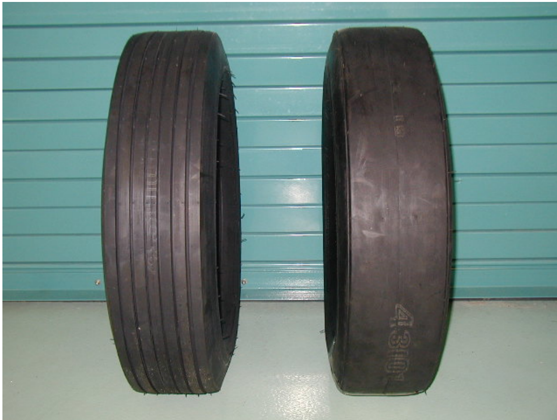
Figure 1 Photographic illustration of a E-501 (ribbed) and E-524 (Smooth) test tire.
