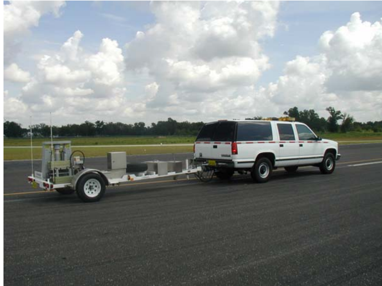
Figure 4. Falling Weight Deflectometer
