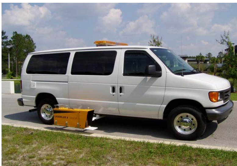
Figure 7. FDOT van with Laserlux attached
