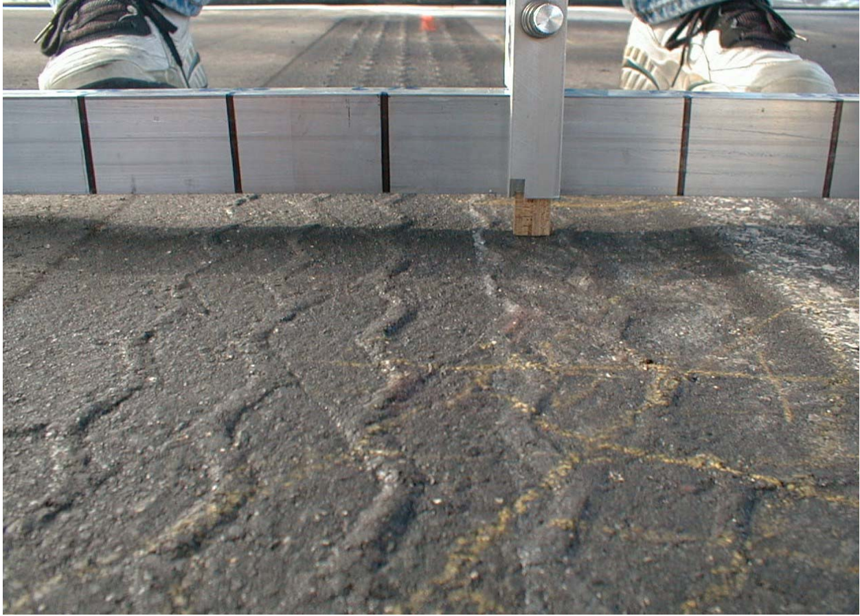
FIGURE 1 Illustration of rut measurement using a straight edge.
