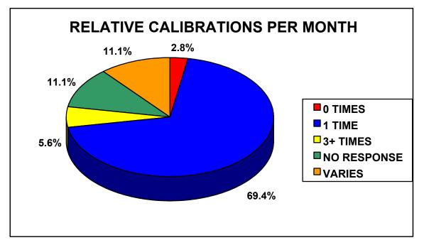
NOTE: Reference Calibration is the calibration of the FWD unit to known reference standards. Relative Calibration is the comparison of FWD deflection sensors to one another.
