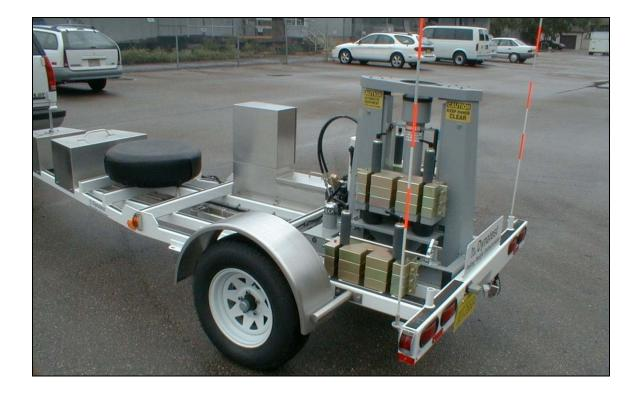
Figure 1 Falling Weight Deflectometer, Dynatest 8000
