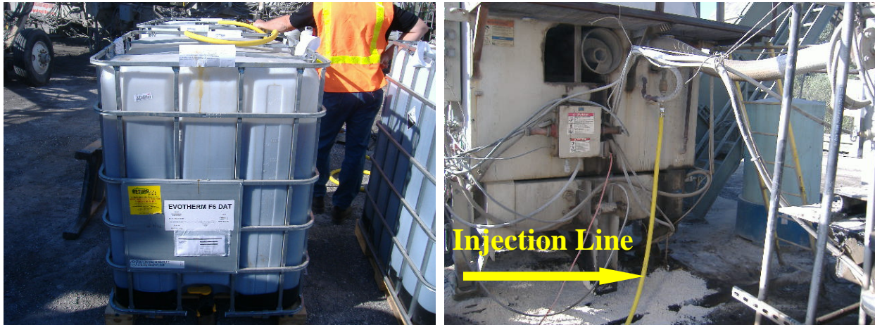
Figure 4 - Evotherm DAT Warm Mix Process
