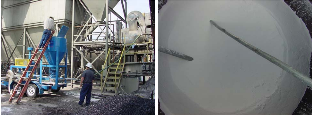
Figure 2 - Aspha-min Warm Mix Process
