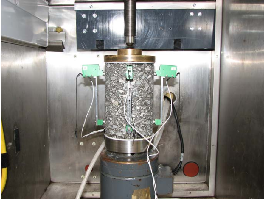
Figure 9. Dynamic Modulus Test
