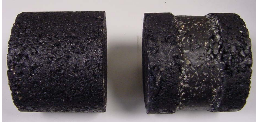
Figure 2. Specimens before and after a RAWT test
