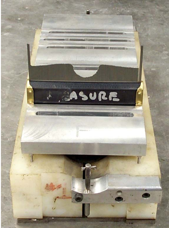
Figure 3-8 Measuring plate and contour gage for modified measuring technique
