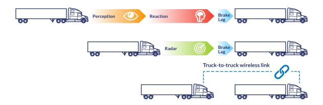
Figure 4: Brake Application Timing w/ Coordinated V2V Operation (Source: Peloton Technology)
