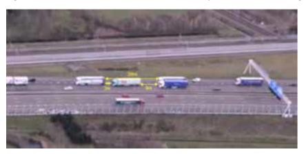
Figure 11: EPTC Overhead Video: Merging Truck Accepts a 3m Headway
