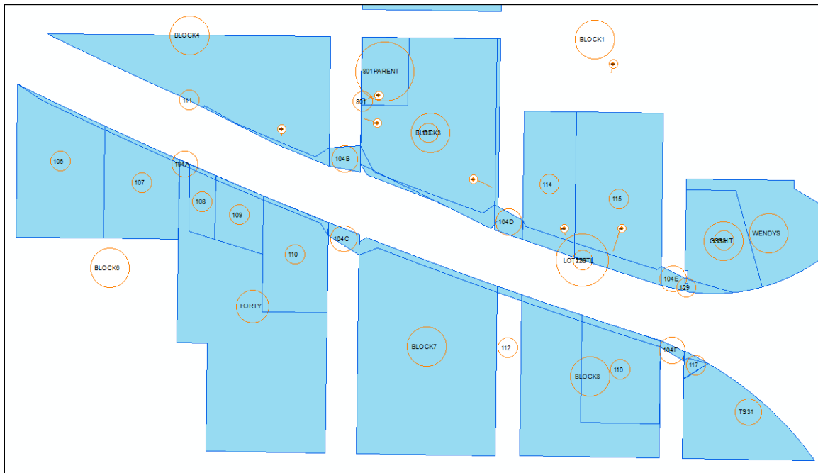
Figure 41. MicroStation GEOPAK Data after Importing Parcels to ArcGIS.
