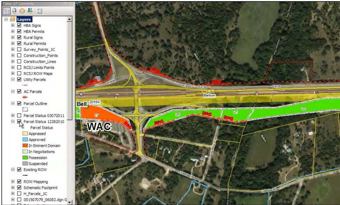
Figure 18. Standalone ArcGIS Tool to Visualize Parcel Acquisition Process (13).
