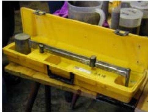
Figure 15, Mud-balance density test equipment
