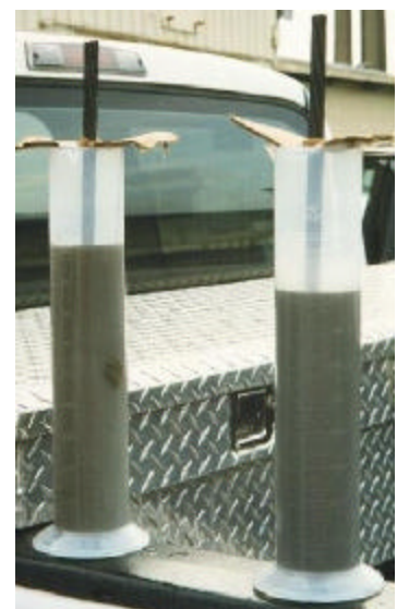
Figure 14, Wick induced bleed tests
