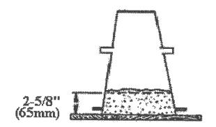
3. Rod the layer with the hemispherical-shaped end of the tamping rod 25 times. Distribute the strokes uniformly over the layer. Rod the concrete to full depth, but don't strike the base forcefully.
