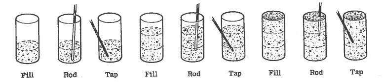
For each cylinder, strike off the excess concrete with the tamping rod using a screeding and rolling motion and level the top of the concrete. Smooth with a trowel.
