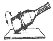
11. Set the meter upright and jar it lightly and allow it to stand until the air rises to the top.
