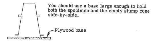
Note: Slump cones need to be held in place by standing on the foot holds.
