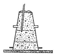
6. Strike off the excess concrete with the tamping rod, using a screeding and rolling motion. Clean excess concrete from around the bottom of the mold.
