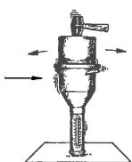
10. With the neck elevated, roll and rock the unit until the air appears to have been removed from the concrete.
