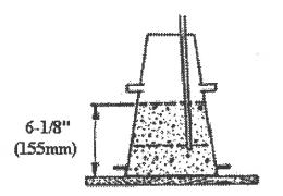
5. Fill the cone to overflowing and rod 25 times, as before. The excess concrete should be above the top of the mold.
