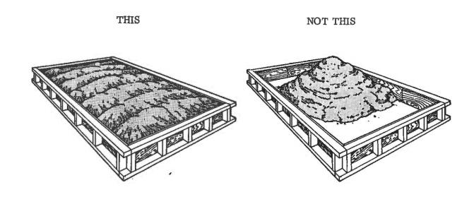
When concrete is being placed in walls or other long, narrow sections, you must be sure that a uniform depth is maintained. Also watch that the layers are not more than 12 inches (300 mm) deep to ensure adequate consolidation. Layers 6 to 12 inches (150 to 300 mm) in depth are about right for easy handling. When concrete is placed on a slope, placement should start at the bottom of the slope.
