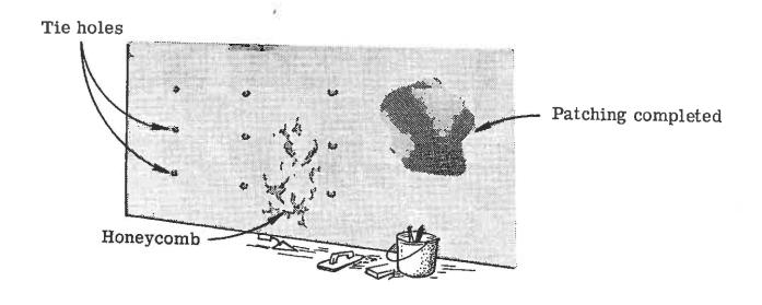
Small areas of honeycomb are repaired by chipping out loose and weak concrete until sound, solid concrete is exposed. Large areas or many small areas of honeycomb indicate that vibration was insufficient during placement. If there is excess honeycomb, the entire section may need to be removed and replaced. You should discuss this with the Project Engineer before repairs are started.
