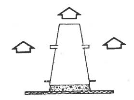
8. Place the tamping rod on the inverted slump cone (extending across the center of the specimen), then measure the difference between the top of the slump cone and the displaced original center of the top surface of the slumped concrete. Measure to the nearest ¼ inch (5 mm).
