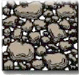
PROPER MOISTURE- moisture helps hold particles together.
