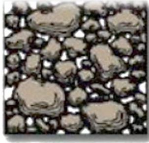
PROPER MOISTURE- moisture helps hold particles together.
