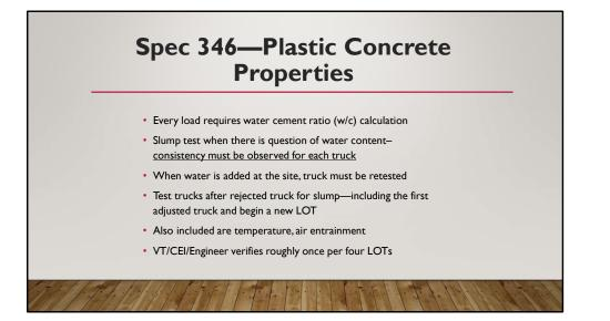
Moving on to Spec 346, (read slide) 30 revolutions after adding water. VT = Verification Testing
