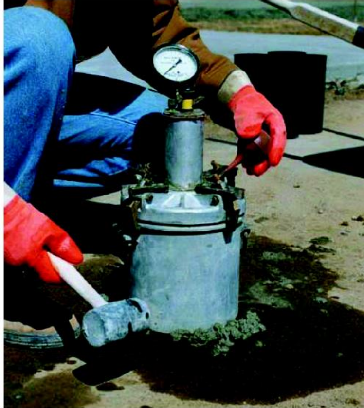
Air Content (Pressure Meter)
