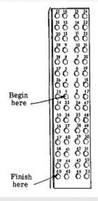
The Sequence of Tightening is <u>CRITICAL</u> →Most rigid, to least rigid
