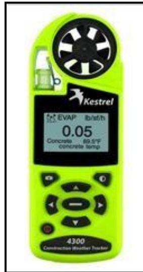
Figure 5 - Weather Meter for Evaporation Rate
