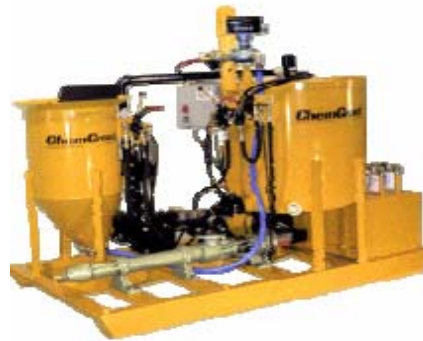
Figure 8, ChemGrout 600 Colloidal grout mixer and pump
