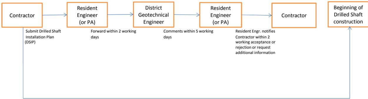
Contractor shall submit DSIP at the preconstruction conference or 30 days prior beginning of drilled shaft construction
