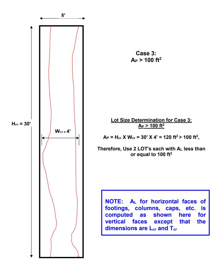
Vertical Face of a Footing, Column or Cap
