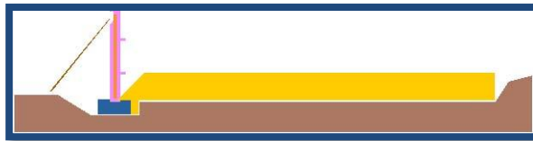
Figure 17-5: Fill in 6" lifts to reinforcement
