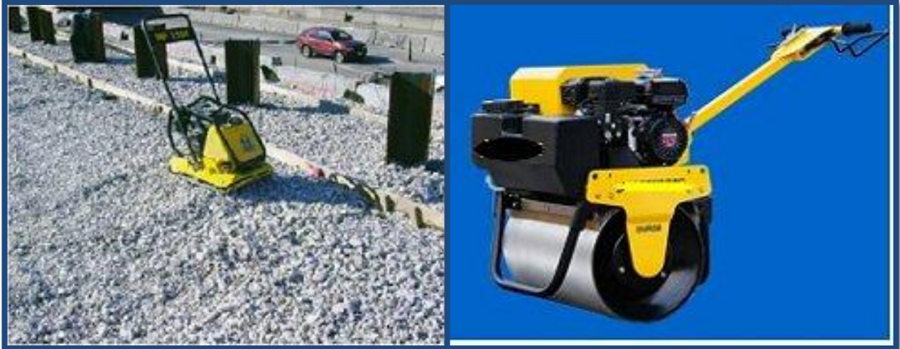
Figure 17-11: Typical Compaction Equipment Used Within 3 feet from the Panel
