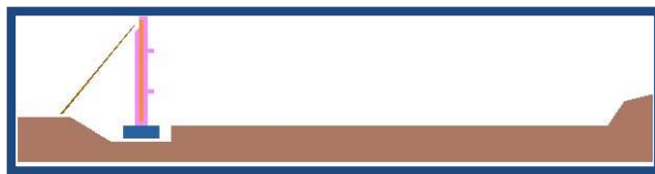
Figure 17-3: Install and Brace First Row of Panels
