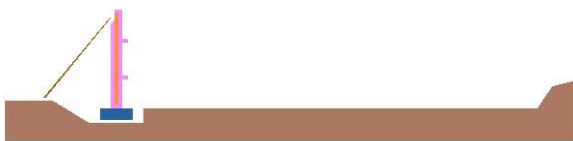
Figure 44, Install & Brace 1st Row of Panels
