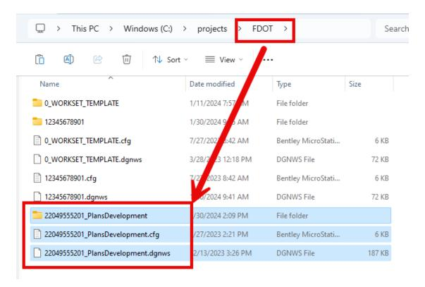
The Training Dataset, including the workset and corresponding .CFG and .DGNWS files associated with the workset, are now located in the *FDOT* subfolder of the *Worksets* folder.
