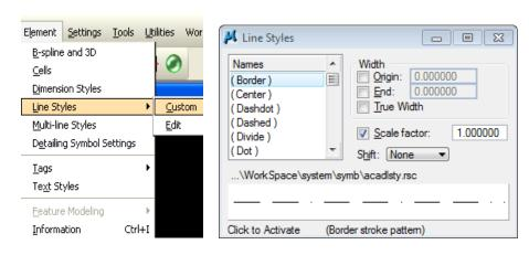
In most instances the MicroStation Custom Line Style name will match the AutoCAD Linetypes, which are defined for AutoCAD in the file *FDOT.lin* located in the \*FDOTXXX.C3D\Support\linetype\* folder.
