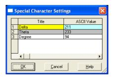
Right of Way project font 58 in MicroStation - If exporting to a Right of Way map, CAiCE needs to be set by selecting the menu items: Settings > Special Characters and set the ASCII value 33 to the Delta symbol as shown in the figure to the right.
