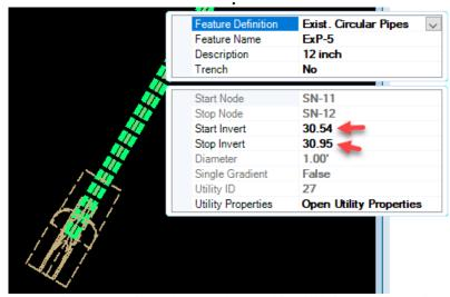
13. To fix the end structures invert elevation select the element this will bring up the handles change the number 31.87 to 30.95
