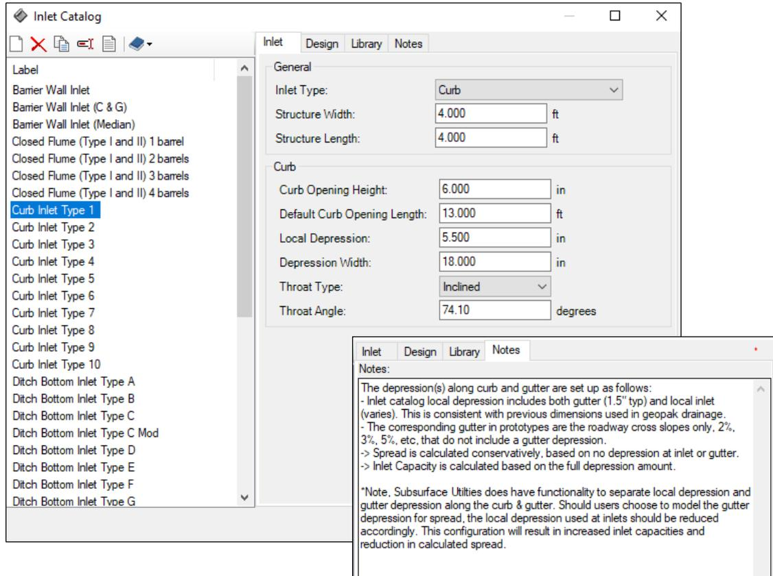
**Note** These parameters are needed for typical FHWA HEC-12 or HEC-22 calculations. The values provided were determined by the Department's staff and are felt to be conservative. Users should verify values prior to performing inlet and spread calculations with Drainage and Utilities Workflow and OpenRoads Designer CONNECT Edition.
