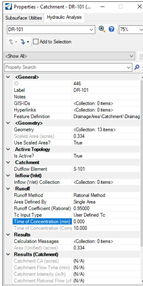
7. There's one more change to DR-101 to better represent the ratio of previous and impervious cover. As an alternative to placing separate shapes for different C values, we're going to edit the properties of DR-101 to calculate the weighted C value. In the Runoff category, select the pulldown for Area Defined By and Select Multiple Subareas.
