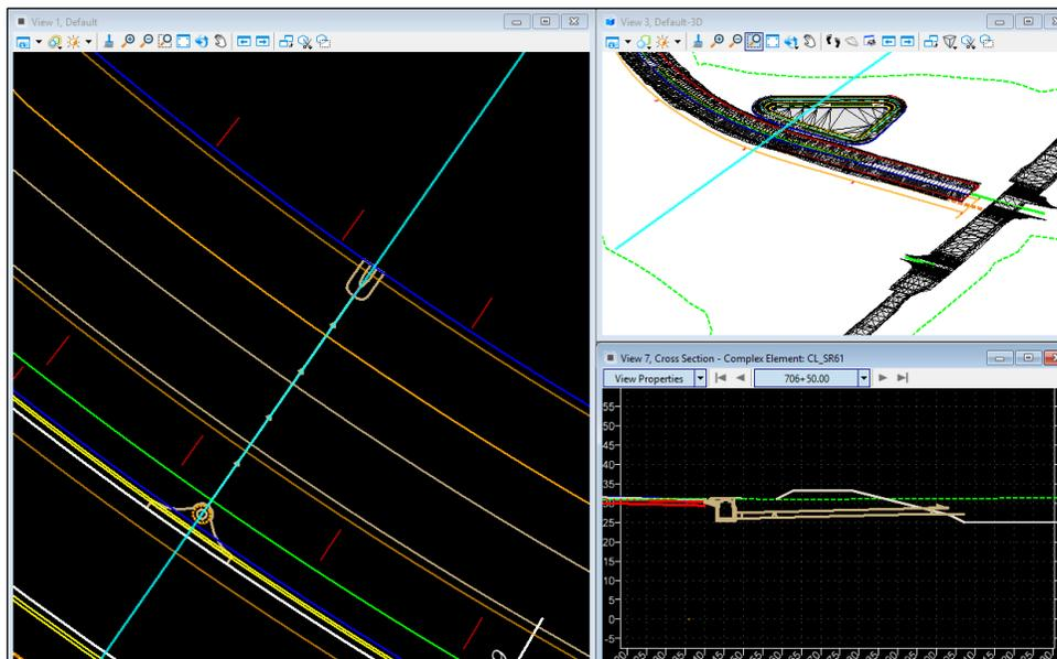
2. Since the MES was placed using a 0.00' vertical offset from the pond surface, the initial pipe invert of P-101 defaulted to the elevation of the pond at the node reference point location. However, now that the S-102 outlet structures is linked to P-101, when we override the downstream invert to EL 25.00, the MES invert elevation will follow.
