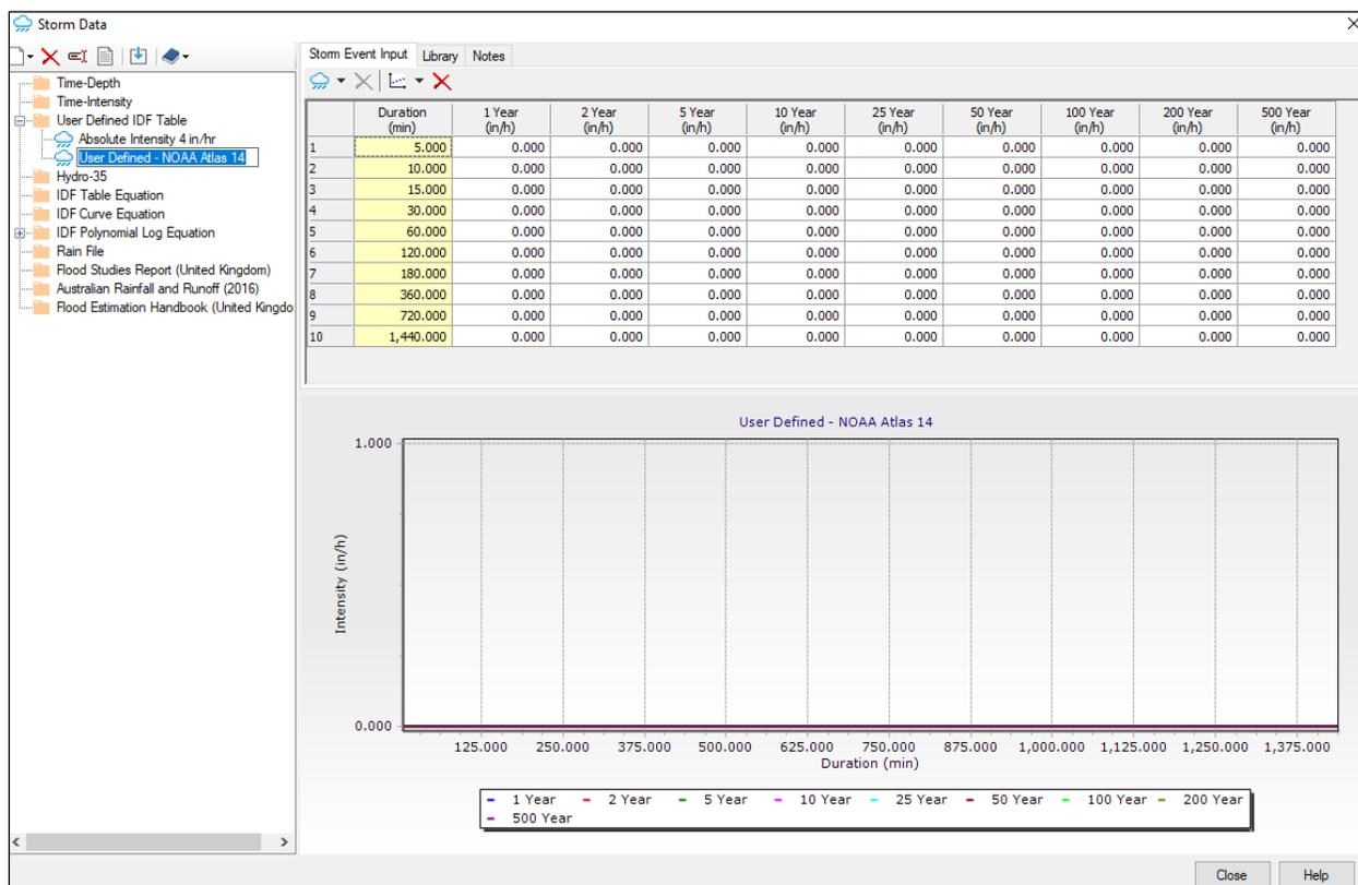
2. By default, the table is empty and set up to receive intensity data for durations 5-min to 24-hr and 1 Year to 500 Year storms.
