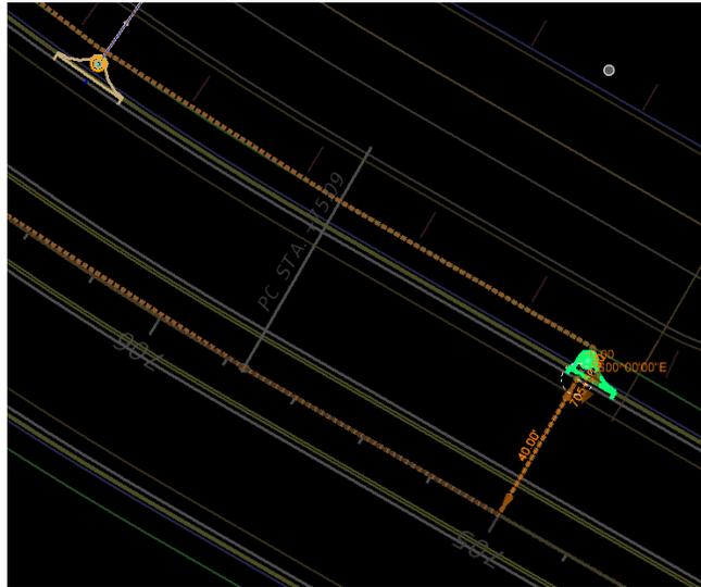
2. Next, use Place Conduit tool to add P-103, a new 18" Circular-Concrete pipe, from S-103 to S-101. Refer to steps in Exercise 2.7 as needed.
