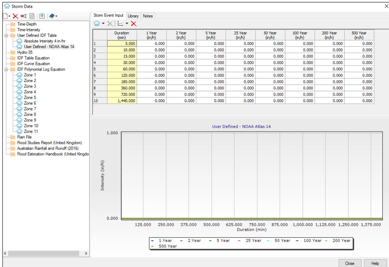
The Absolute Intensity IDF Table includes a constant 4 in/hr intensity for spread analyses.
