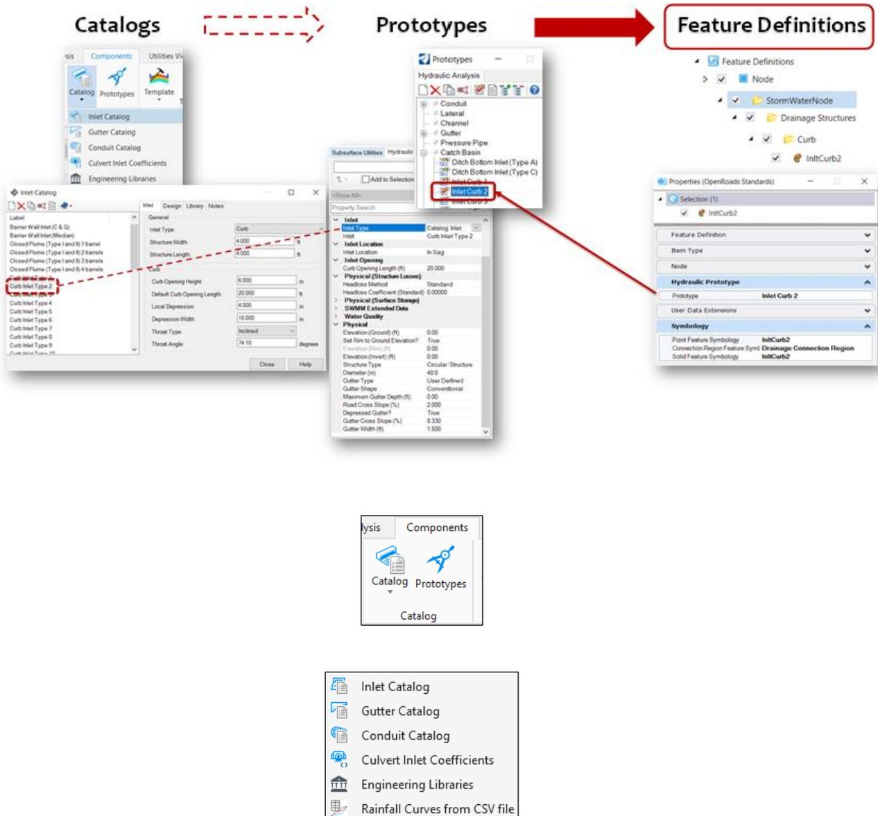
The catalog windows contain several tabs to define input, design parameters, engineering library connections, and notes. Where applicable, notes have been included to clarify input. Though FDOT inlets do not have variable opening lengths subject to design, the conduit catalog is built so that automated design selects from available standard pipe sizes
