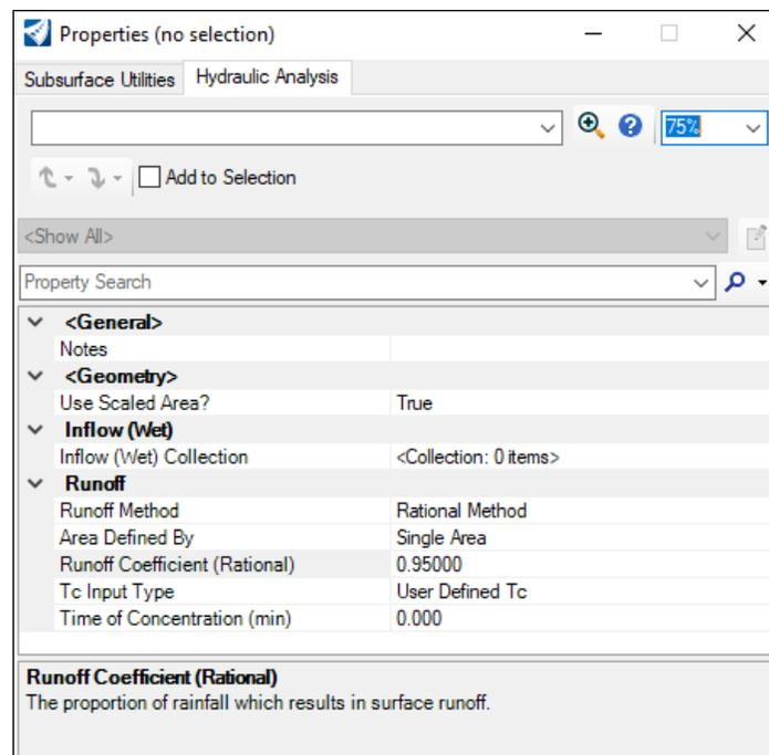
2. Since this is a prototype, settings shown in this **Properties** dialog are applied by default to new catchments with feature definition = Pavement. For Pavement, the assigned C value is 0.95. Time of Concentration is set to user defined, which can be assigned after placement. Close the properties dialog.
