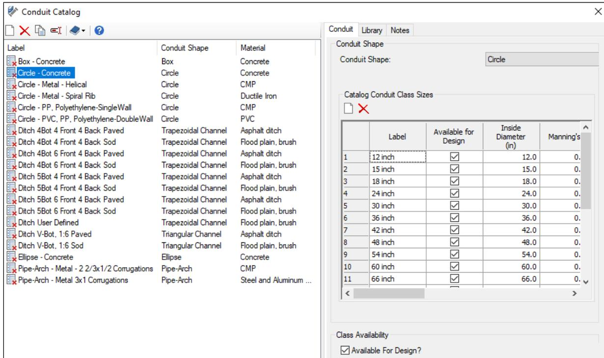
**Note** Conduit vs. Gutter: Conduits model system flow that is intercepted by and passed through nodes. Gutters model bypass flow along the ground surface between nodes. Open channel ditch shapes are included in each catalog with the FDOTCONNECT Workspace.
