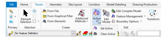
4. At the cursor prompt, select the **Terrain Boundary** green dashed line from the attached *SURVRD01* reference file. This will set the terrain model as active.
