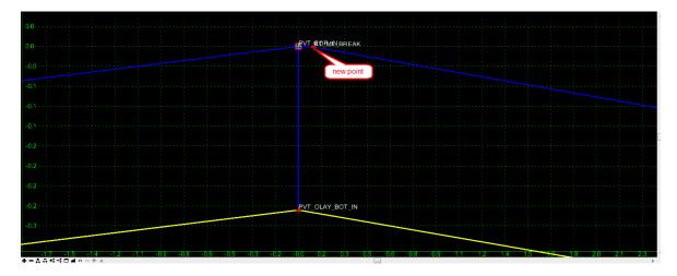
5. Repeat the steps above to insert *Points* on the bottom of the **PvtOverlay**, **PvtMilling**, and **PvtOverbuild** *Components*.
