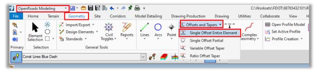
13. Single Offset Entire Element from the End Bent Cap 2.67' to represent the front face of the MSE Wall offset from the End Bent Cap. Offset will vary depending on project and must maintain minimum clear as required by the FDOT Structures Design Guidelines.
