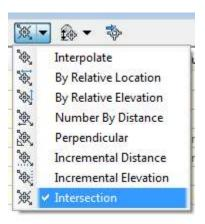
Creating Alignment by Layout instead of Object eliminates the step for polylines. Result is the same as when you create an object and as easy.
