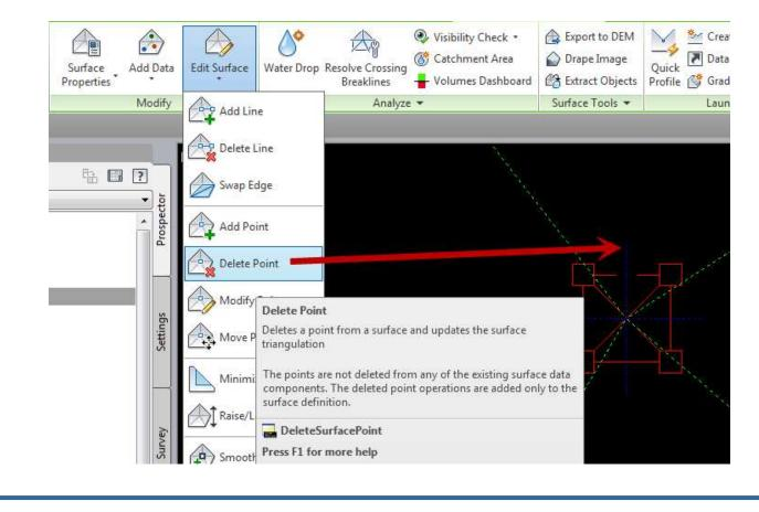
To delete a surface point vertex: from the ribbon select the "Edit Surface" drop down and select "Delete Point". Press enter to complete the deletion.
