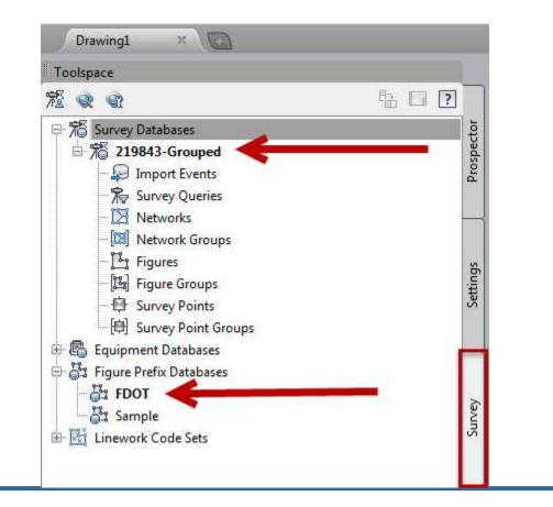
To populate the survey database with an XML file from CAiCE or EFB, right click on the Survey Database name and select Import and choose "Import survey data..." (import wizard) or "Import Survey LandXML...".
