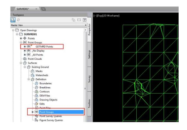
In the Toolspace>Survey tab, right click on the GDTMRD Chains figure group and select "Create breaklines...".
