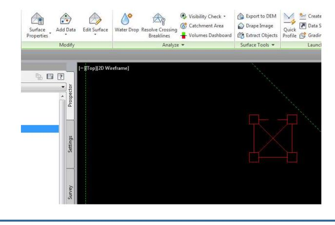
Additional edits can be made from the "Edit Surface" drop down such as "Delete Line" to remove a triangle and "Add Line" to add a triangle.
