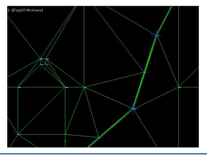
To delete a surface point vertex: from the ribbon select the "Edit Surface" drop down and select "Delete Point". Press enter to complete the deletion.
