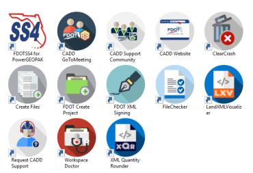
Using these shortcuts to start the applications will provide the designer with the environment properly set with the FDOT CADD standards. The FDOT delivers shortcuts for starting PowerGEOPAK, MicroStation or MicroStation with GEOPAK Suite depending on the registry configuration.
