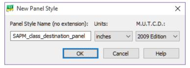
**Note** A panel style represents a set of parameters that specify the characteristics of a sign (sign shape, color, border radius, thickness, fonts, size of arrows and shields, and spacing between text and symbols). The highlighted panel style is used to create new panels.
