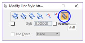
11. Select one of the shorter lines of conduit. Move the cursor to shift the lines style so that the dots of the custom line style appears and **data point** to shift the line.
