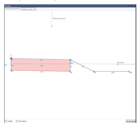
15 Drag and drop a Point from the Geometry section on the Toolbox under the point and link previously created. On the Properties panel, under Point Geometry Type, select Slope to Surface. Under Point Geometry Properties, select From Point P10 and type in CutSlope for Slope, set the Surface Target to EG, and turn on under Link, Add Link to From Point:
