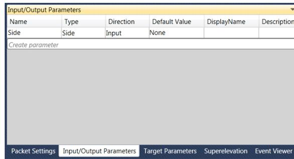
If now, the width of the shape is to be controlled not by a target parameter, but by an input/output parameter, they must be defined on this window.
