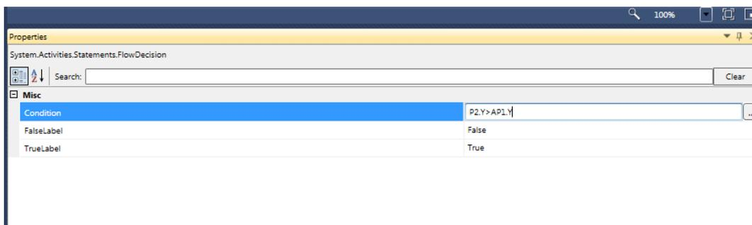
**Note** This condition rule will be true if point P2 is above the existing ground point, AP1 (Fill Condition)
