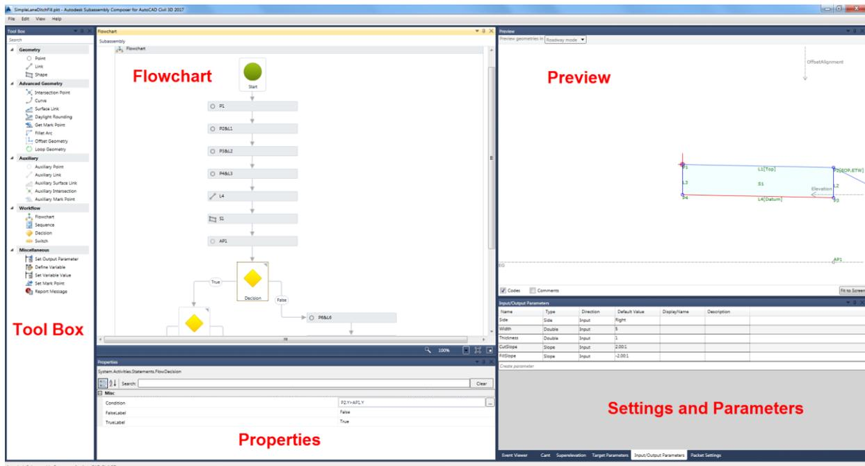
The Toolbox window is the storage location for elements available for constructing the subassembly. This window will provide all elements used to build the flowchart. There are five sections: Geometry, Advanced Geometry, Auxiliary, Workflow and Miscellaneous. To use any of these elements, simply click on the desired element and drag and drop it over into the Flowchart panel.
