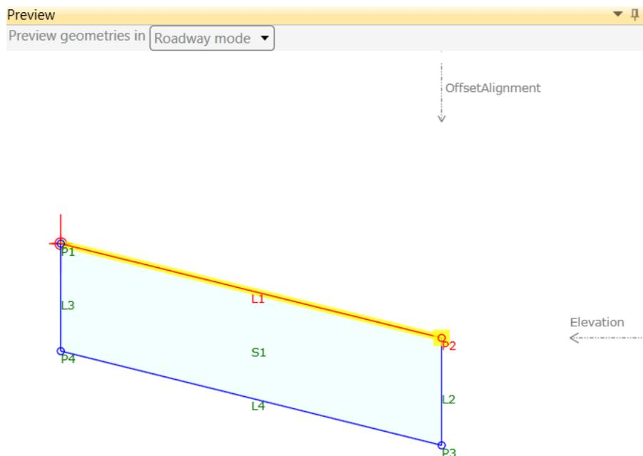
If these targets are defined in the Corridor in Civil 3D, the width and slope of the link will be controlled by an alignment and Elevation Targets.
