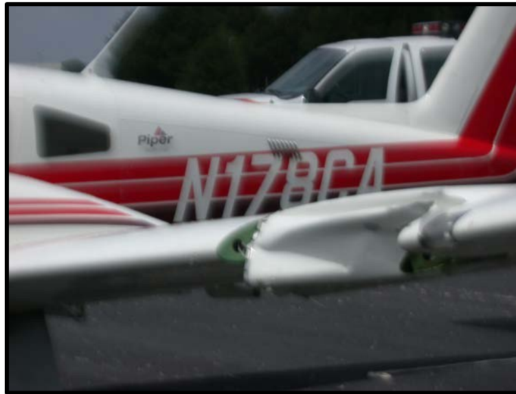
FIGURE I-2 BIRDSTRIKE DAMAGE TO PIPER SEMINOLE DURING LANDING APPROACH TO A FLORIDA AIRPORT (MARCH 2003)
