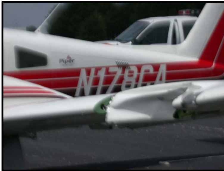
FIGURE L-2 BIRDSTRIKE DAMAGE TO PIPER SEMINOLE DURING LANDING APPROACH TO A FLORIDA AIRPORT (MARCH 2003)
