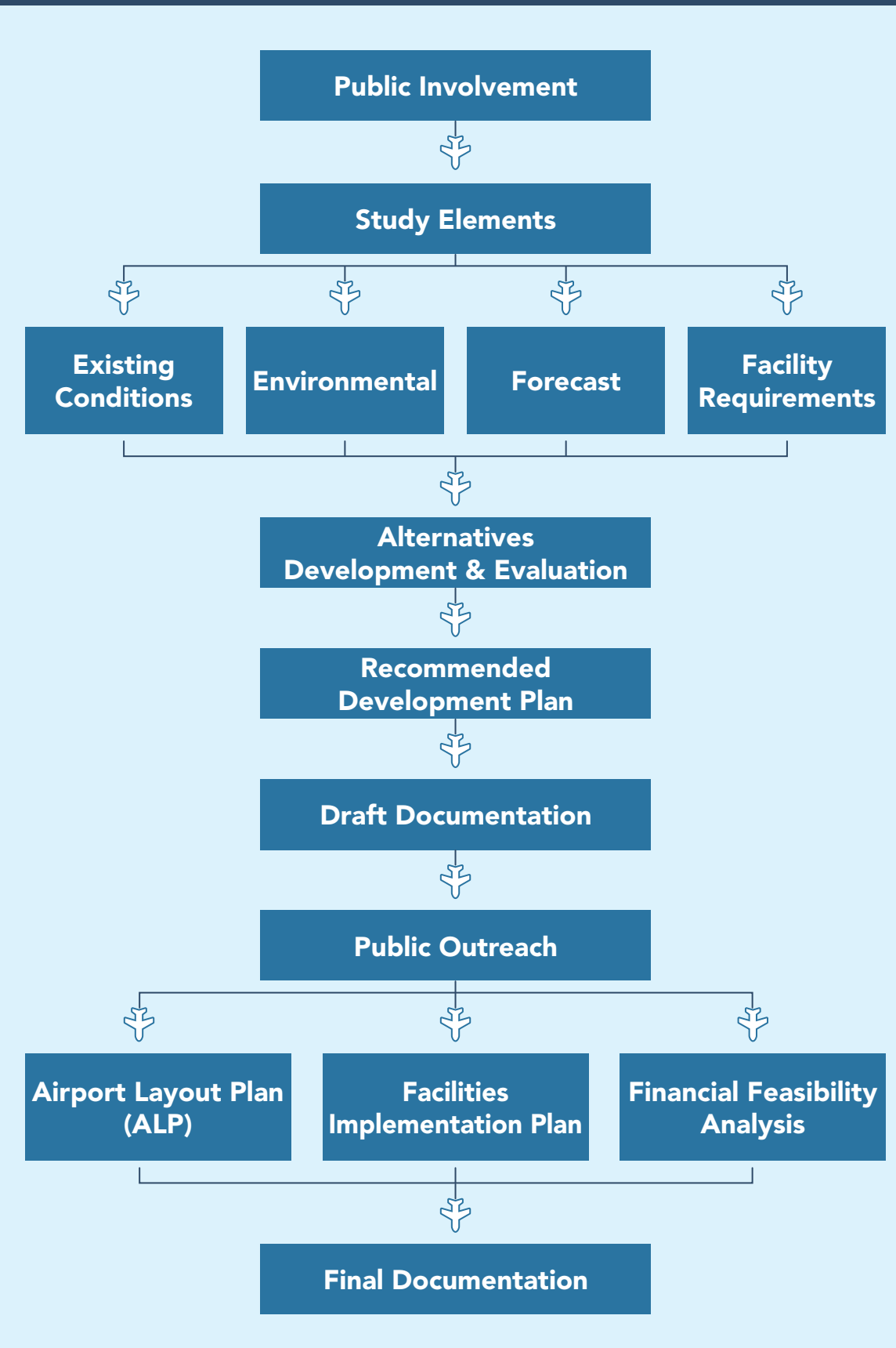
FIGURE 5. AIRPORT MASTER PLANNING PROCESS
